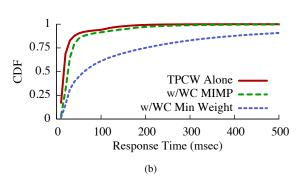
Figure 6. The MIMP scheduler provides response time almost equivalent to running a web application alone.
