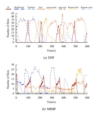
Figure 10. The slot allocation for the first 10 minutes - MIMP vs. EDF
