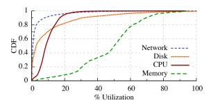
Figure 3. Servers used to host VMs for our IT department illustrate that many resources are often left idle; memory is the only resource with a median utilization level above 50%.
