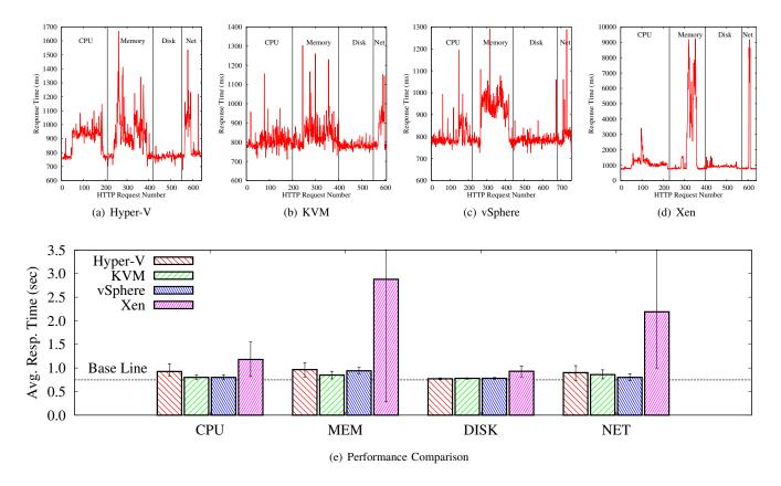
Fig. 9. Interference Impact for Web Requests: 4 VMs (1 web server, 3 workload generators) are used. 3 VMs run the same workload at the same time. The workloads run in the sequence of CPU, memory, disk, and network workloads over time span. We can easily identify 4 interference sections from each graph.
