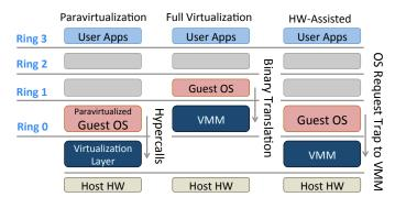
Fig. 2. Different Approaches to Providing the Virtualization Layer
