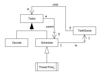
Figure 2.1: Data Model of the Scheduling System
