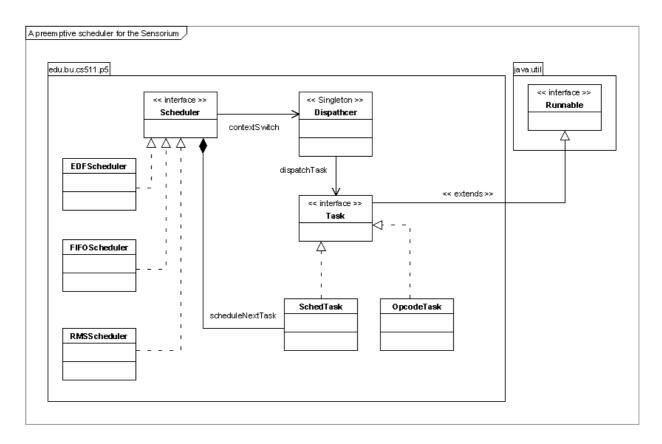
Figure 6.1: UML diagram of the initial Preemptive Scheduler
