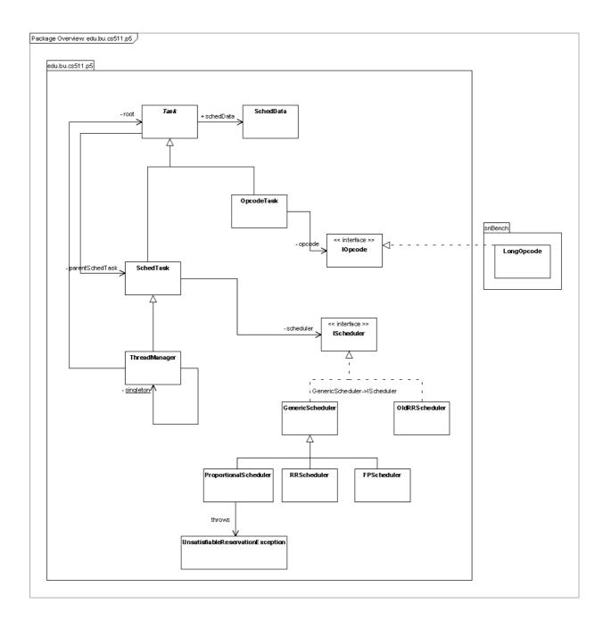
Figure 3.1: The UML Diagram of the Scheduling System
