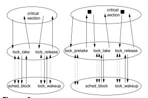
**Figure 2.** Invocations made between components for the pessimistic and optimistic algorithms assuming contention when taking and releasing the lock. *Left:* pessimistic lock component. *Right:* optimistic lock library and component. Dotted invocations designate invocations of sched\_comp\_critsect\_take and sched\_comp\_critsect\_release. The black square indicates atomic instructions.
