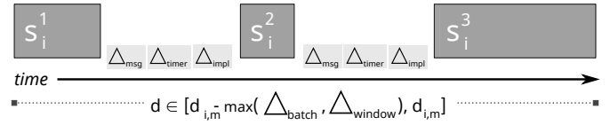
Fig. 5: A timeline of processing a packet through stages s_i^1, \dots, s_i^3 . In between stage computation, maximum system overheads for MMA processing ( \Delta_{\text{msg}} ), event notification triggered by frequent timers ( \Delta_{\text{timer}} ), and scheduler implementation ( \Delta_{\text{impl}} ), impact end-to-end latency. The deadline used by the scheduling logic (including priority inversion) for the end-to-end processing of each message/packet, d , is bounded by batch and timer window size.
